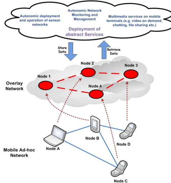
Fig. 1. Proposed approach for autonomous and decentralized services in the IoT
